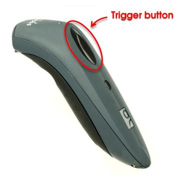
Note: The Bluetooth scanner is slightly different than the scanners we use. When you scan, the red laser disappears then the scanner vibrates and beeps when the info hits the tablet. This can feel slightly delayed.
